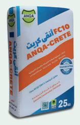
**ANQA-CRETE FC10** is a cement mortar composed of high-strength hydraulic binders, silica sand, selected aggregates, special additives and synthetic fibers, supplied indry, ready-to-use powder blend which requires only addition of clean water to produce easily workable mortar with thixotropic effect. ANQA-CRETE FC10 can be applied to vertical surfaces without sliding even for thick layers.
